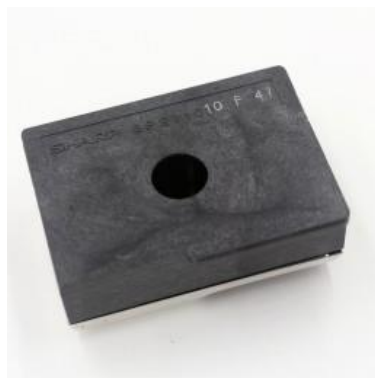
Figure 6: The Sharp optical dust sensor
